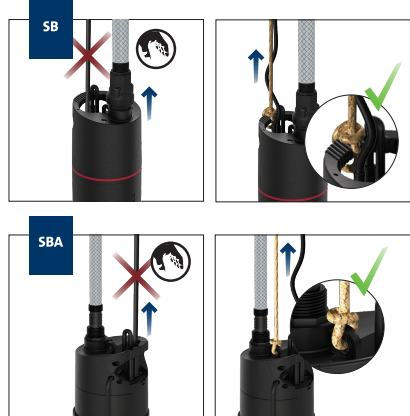
Lifting the pump
