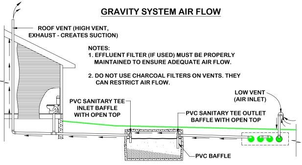
VENTING IS ESTABLISHED THROUGH SUCTION (CHIMNEY EFFECT) CREATED BY THE DRAW OF AIR FROM THE HIGH VENT, WHICH DRAWS AIR INTO THE LOW VENT AT THE LEACH FIELD THEN THROUGH THE SEPTIC TANK AND EXHAUSTED THROUGH THE (HIGH) ROOF VENT.
